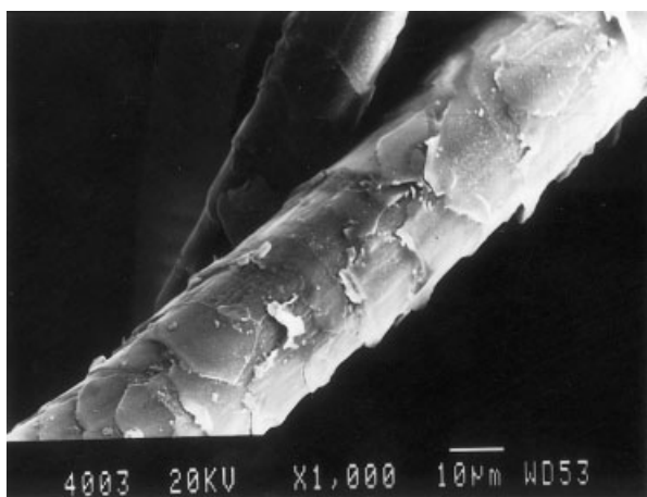
Figure 1 Scanning electron micrograph of a control wool fiber.
